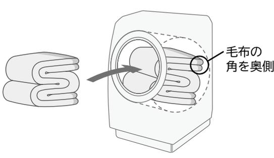
The diagram shows the folded blanket being placed into the drum of a washing machine. A callout points to the back corners of the blanket with the text "毛布の角を奥側" (Place the corners of the blanket to the back).
